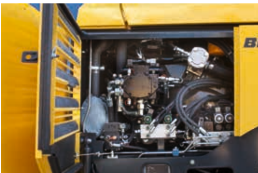
Easy access to: - central hydraulics - pumps - valves - connections
