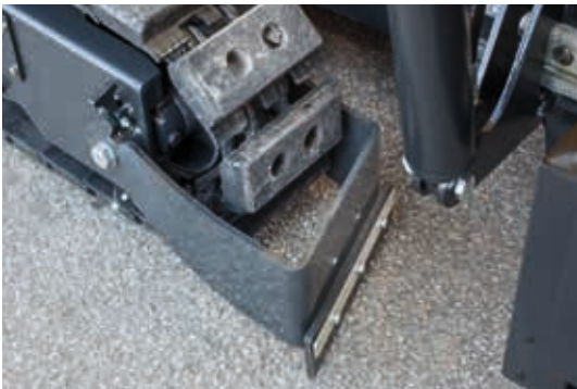
Ensures that the track trains have a smooth contact surface – the sturdy scraper.
